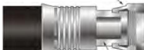
Swivel joint sensitive to over-torquing
